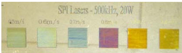
Figure 1: Colour marking, on titanium, showing colour variation based on changing marking speed.
