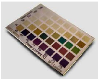
Figure 2: Colour swatches, on stainless steel, made at 125 kHz showing the effect of scan speed and average power – marked with an SPI fiber laser.
