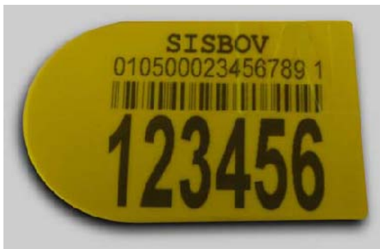
Plastic marking of cow ear tags Polyurethane, with an absorber, marked in 6.7s at an average power of 20W and waveform 0 (25kHz).
